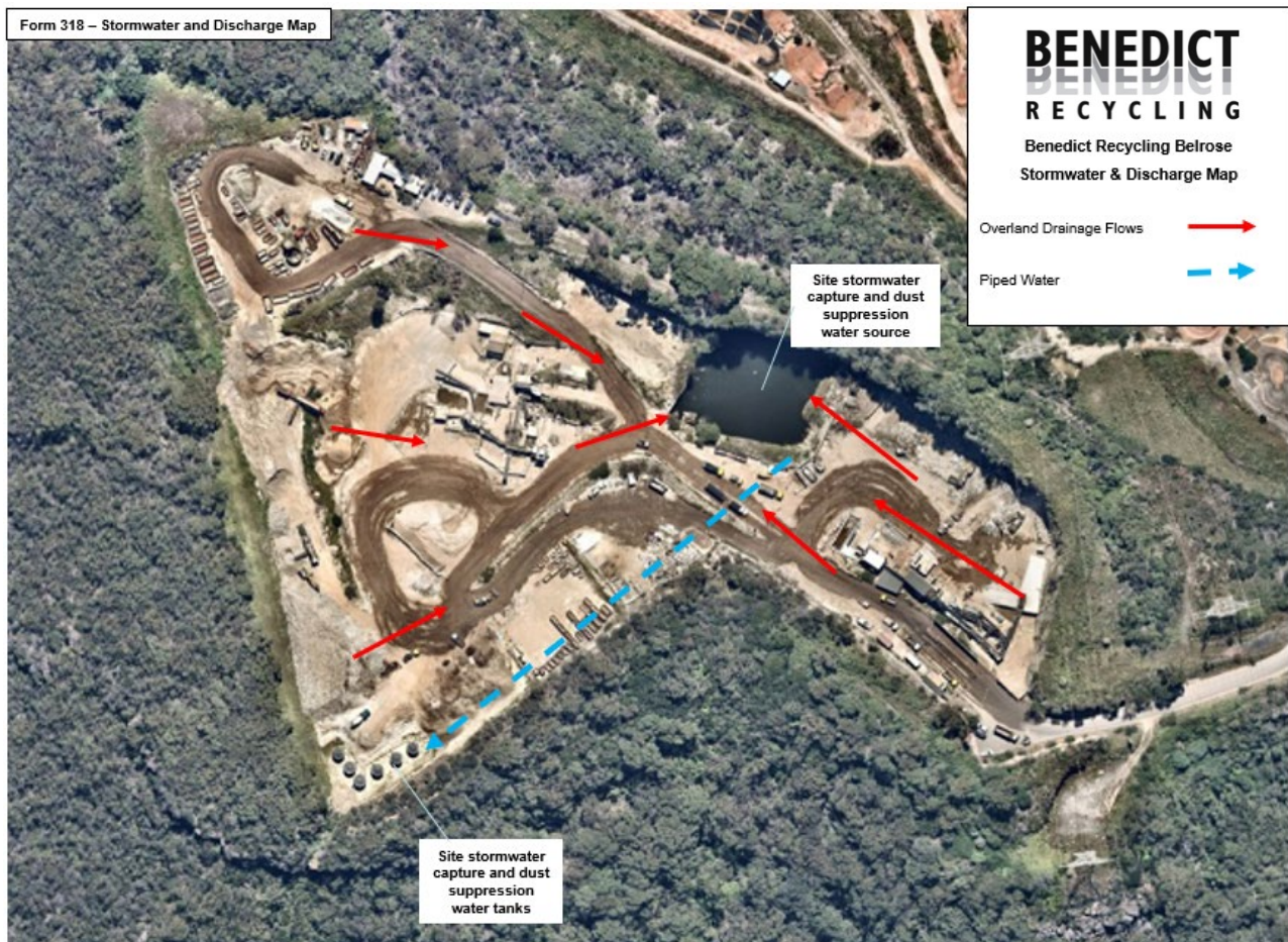
Figure 2: Site Stormwater Directional Flows
