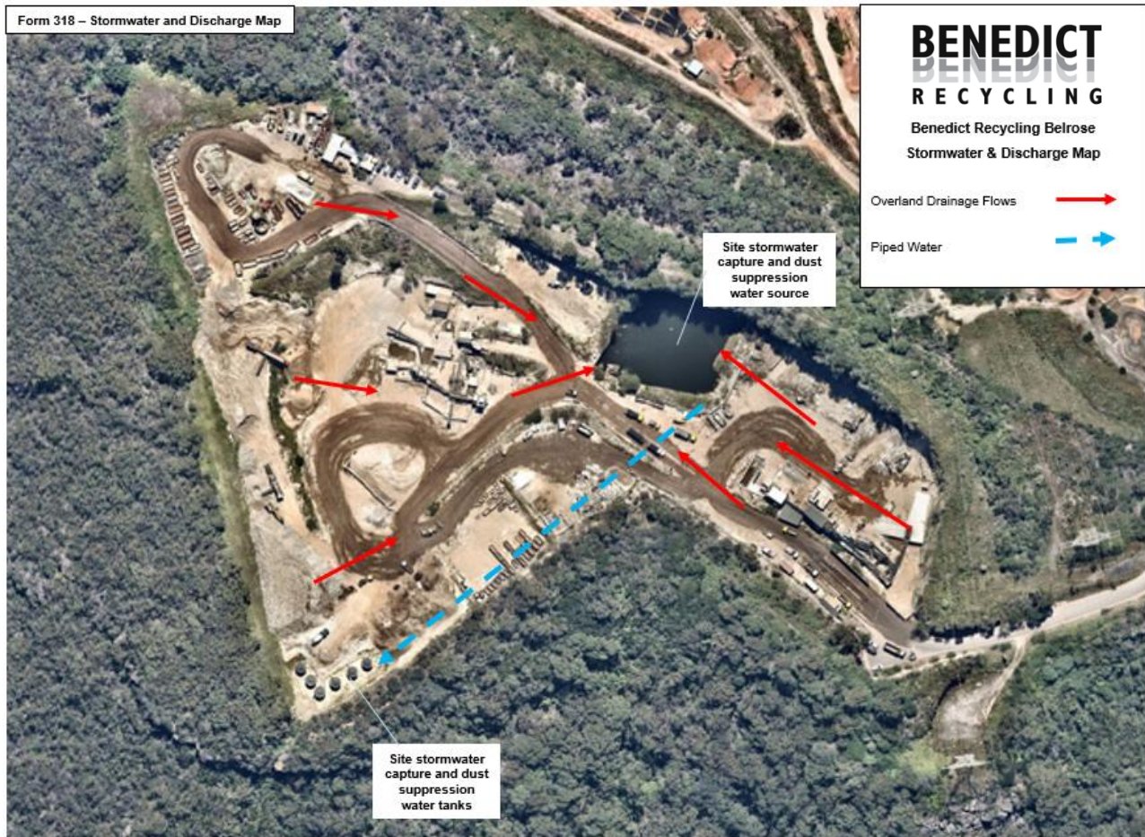
Figure 2: Site Stormwater Directional Flows
