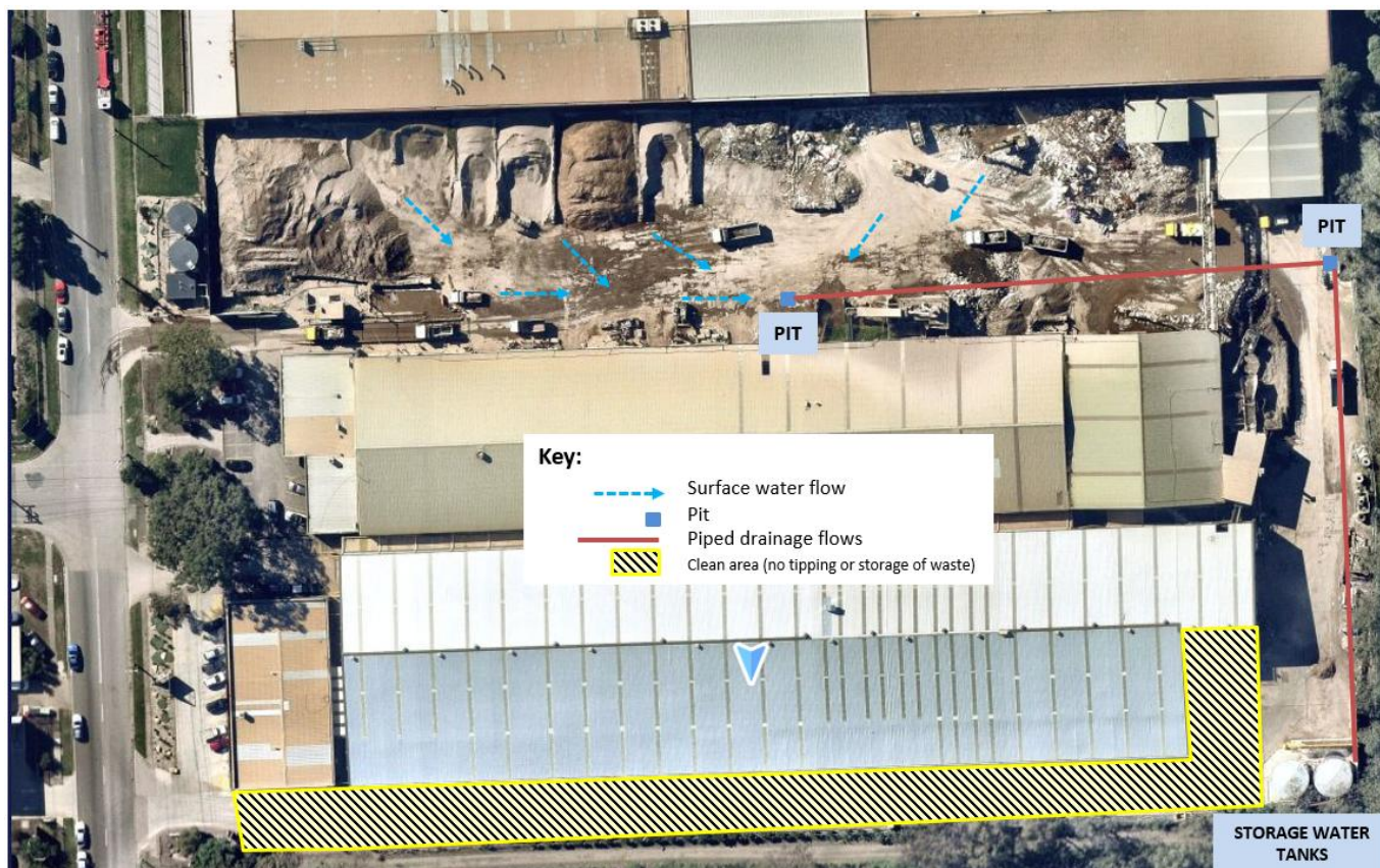
Figure 2: Site Stormwater Directional Flows
