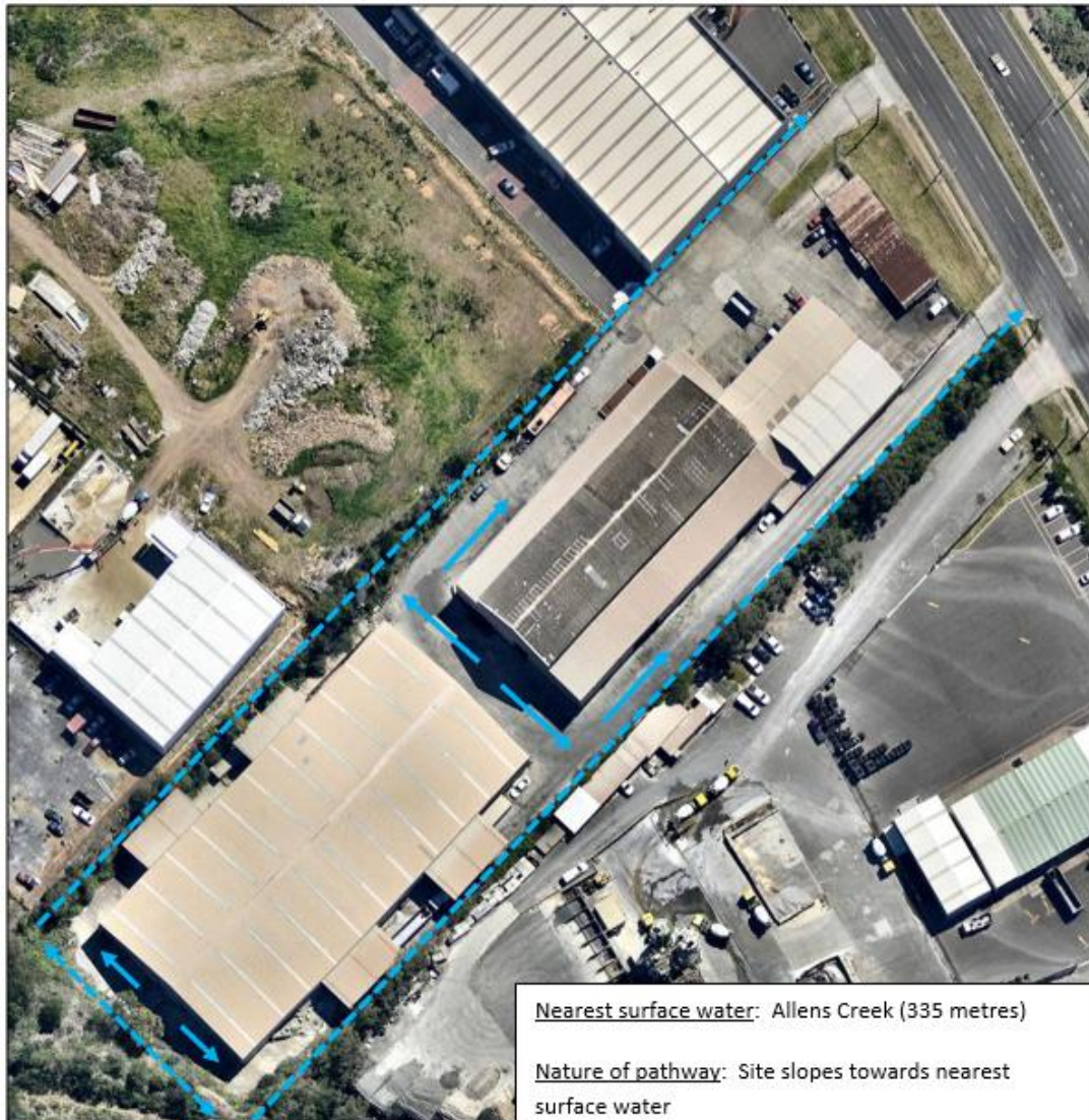
Figure 2a: Site Stormwater Directional Flows
