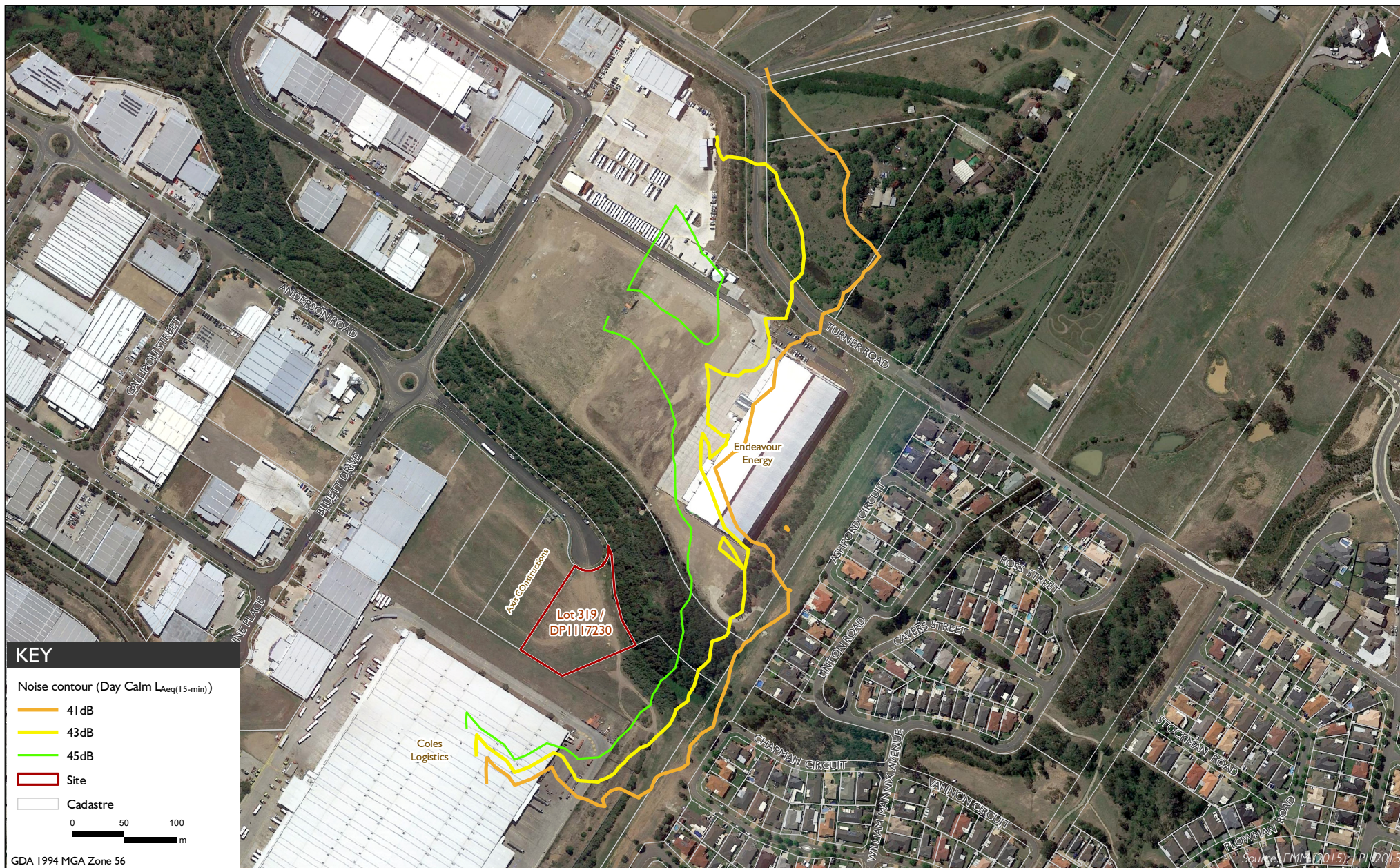
Predicted operational noise contours – Day Calm L_{Aeq}(15\text{-min}) Smeaton Grange Recycling Facility Noise Impact Assessment Figure B.1
