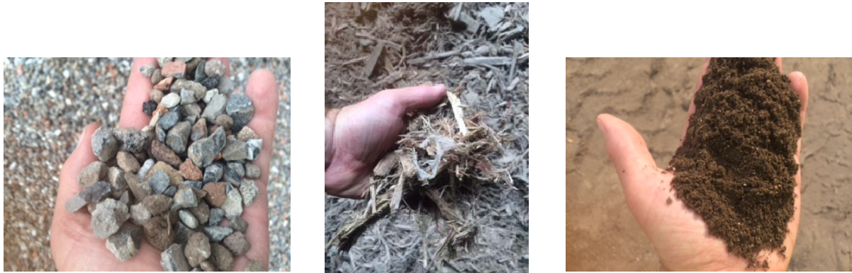
Photograph 2.3 Examples of ready-to-use products (left-to-right: building aggregate, shredded timber and soil substitute)
